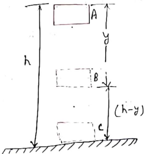
In figure consider a body just dropped on the ground from position A to ground C.
