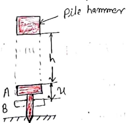
A pile and pile hammer is shown in the above figure. The pile hammer has potential energy before released. After release, the potential energy is converted into kinetic energy, with which the hammer will strike the pile.
