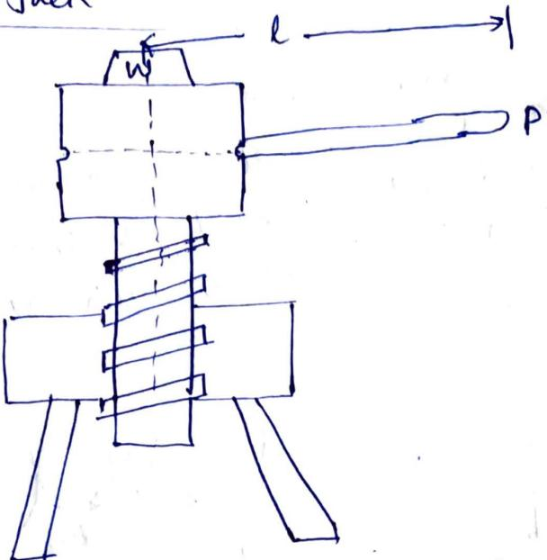
Fig shows a simple screw jack, which is rotated by the application of an effort at the end of the lever, for lifting the load.
