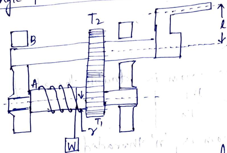
A rope is fixed to the drum and is wound round it. The free end of the rope carries the load  $W$ .
