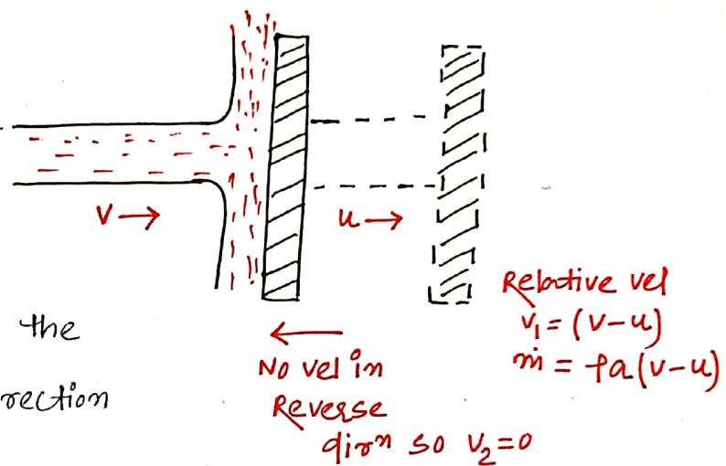
Force Exerted by the Jet on the moving plate in the Jet direction
