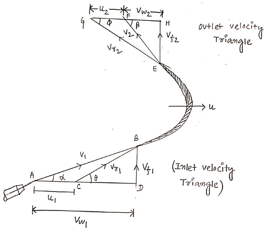
$v_1$  = Velocity of Jet at Inlet.
