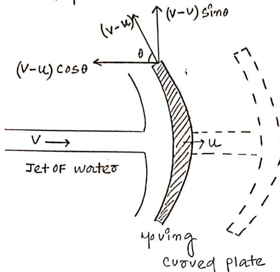
$F_n = m \times \text{component of vel. in the dir}^n \text{ of Jet (Initial - Final)}$
