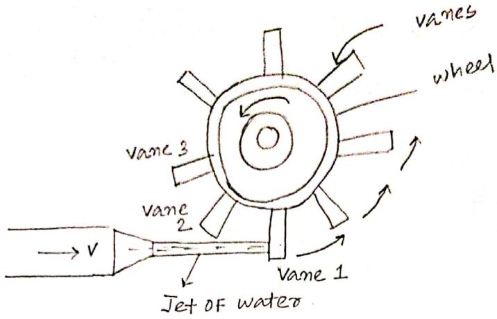
when the Jet strikes on the plate and due to the force exerted by the Jet on the plate the wheel starts rotating.
