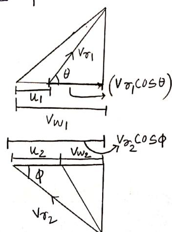
Force Exerted by the Jet in the direction of motion
