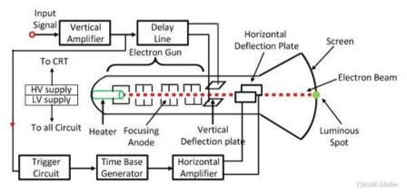
After moving the control grid the electron beam passing through the focusing and accelerating anodes. The accelerating anodes are at a high positive potential and hence they converge the beam at a point on the screen.
