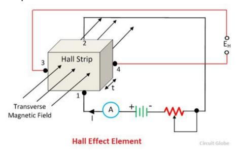
When the magnetic field is applied to the strip, the output voltage develops across the output leads 3 and 4. The develops voltage is directly proportional to the strength of the material.
