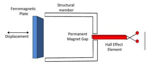
Measurement of Displacement Using Hall Efect Transducer
