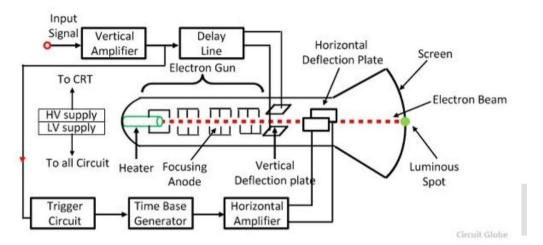
After moving the control grid the electron beam passing through the focusing and accelerating anodes. The accelerating anodes are at a high positive potential and hence they converge the beam at a point on the screen.
