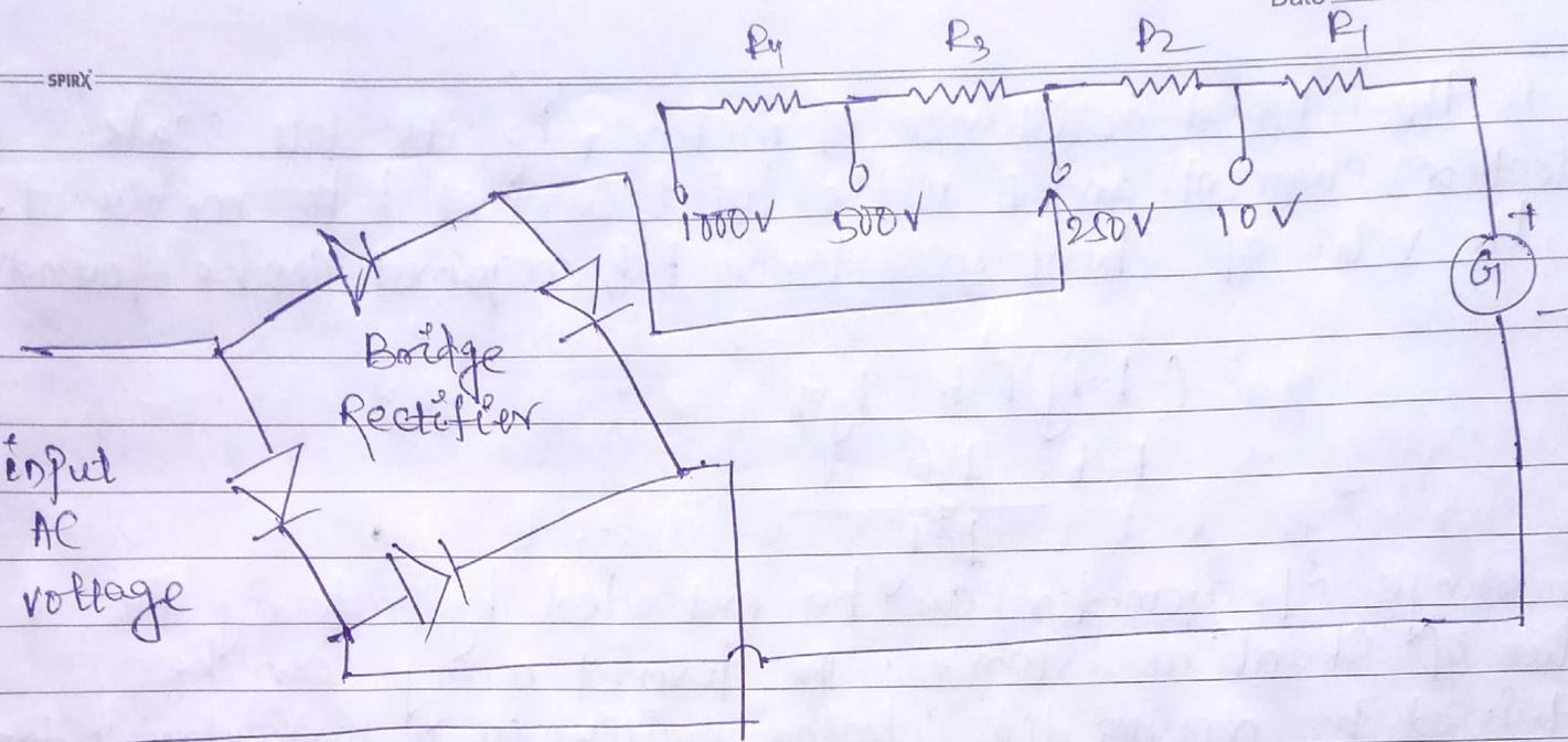
**Current  $M_v$**  → while using Analog multimeter as a voltmeter it must be connected parallel with the portion of the circuit across which the voltage is being measured.
