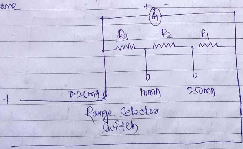
If 'G' is the internal resistance of meter,  $I_g$  its full scale deflection current and 'I' is the total current to be measured, then the value of shunt resistance  $R_{sh}$  required can be found as
