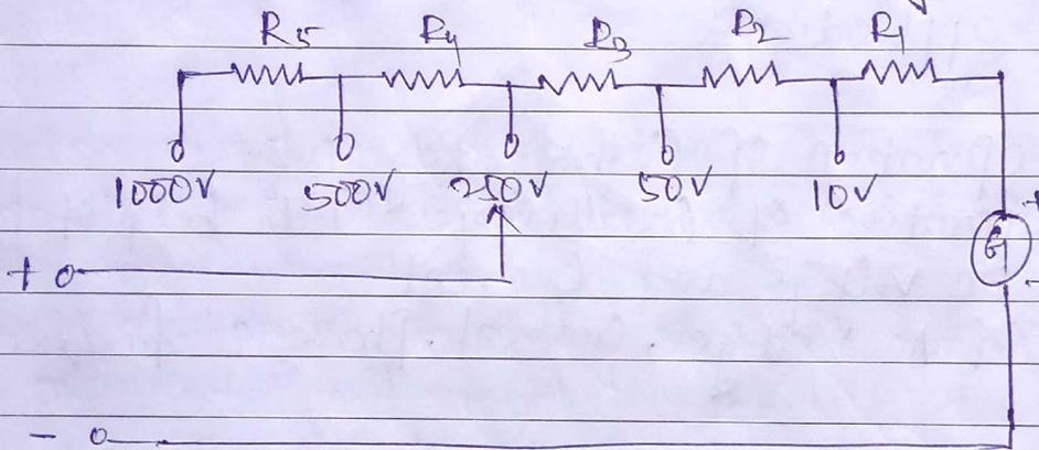
If the Galvanometer resistance is denoted by 'G' and \$I\_g\$ is the full scale deflection current and the voltage to be measured is 'V' volts, then the value of series resistance '\$R\_s\$' is determined as
