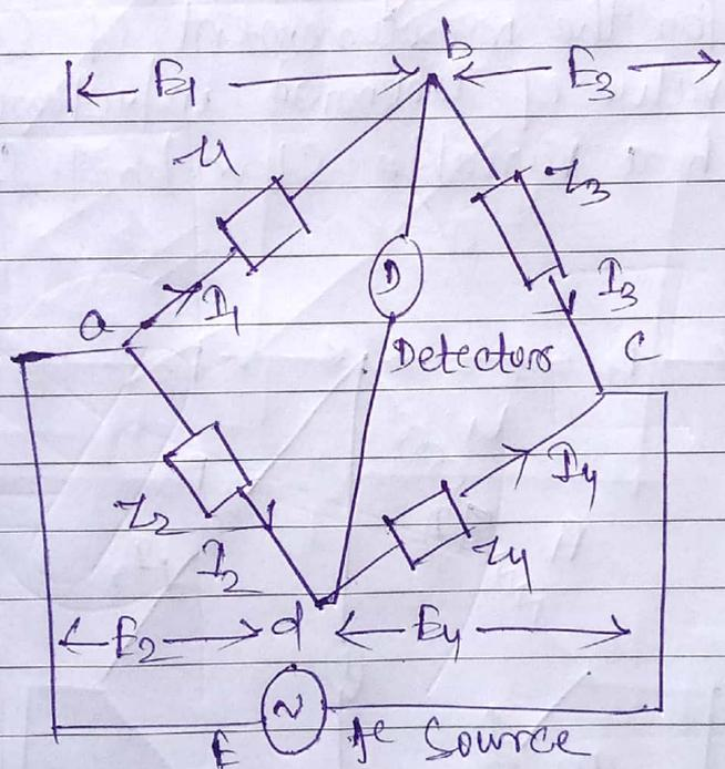
At balance condition, no current flows through the detector. Thus  $I_1 = I_3$  and  $I_2 = I_4$  which means potential across point 'b' and 'd' are equal.
